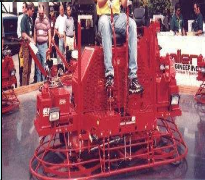
Finishing Rotary Power Trowel (Rider - Double Blade)
