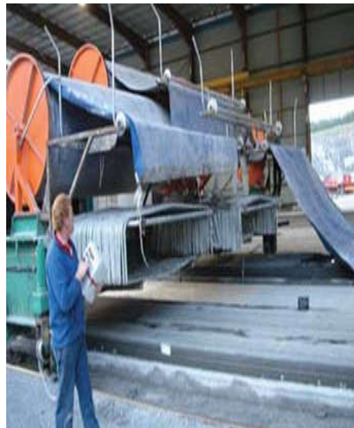
Tarping process for vapor curing of hollow core planks
