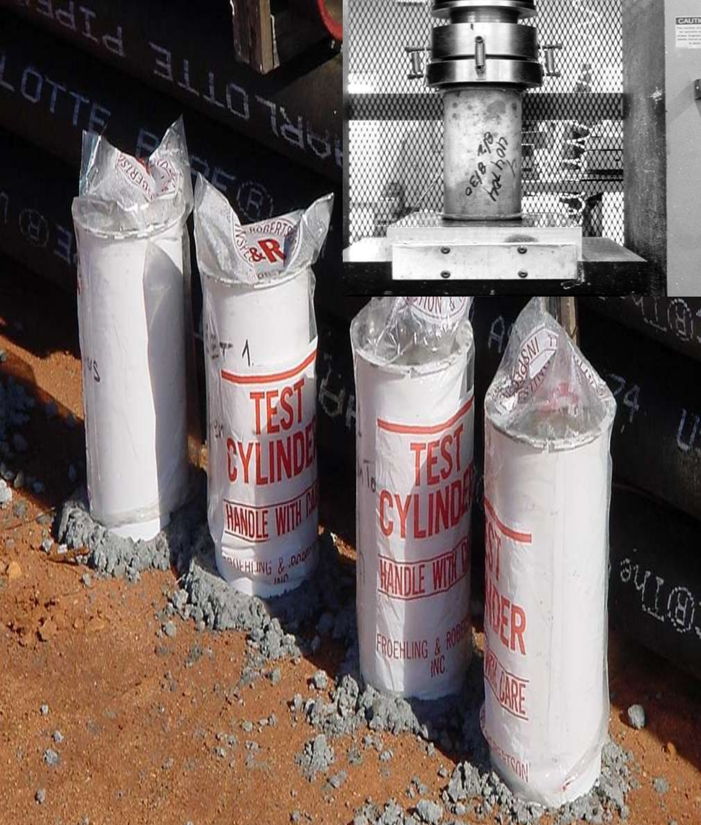
Test Cylinders Curing and then strength tested (upper right)
