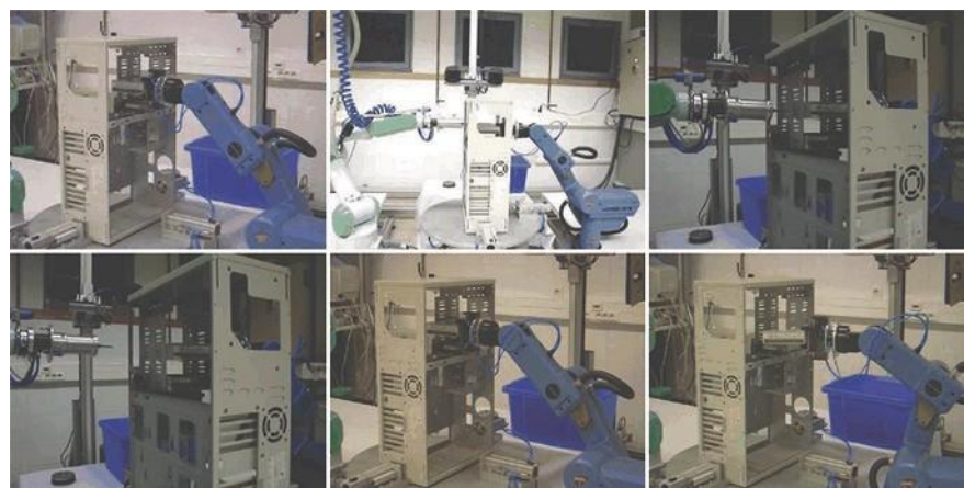
Fig. 3.15 Multi-sensorial cooperative robots—demonstrate removing CD drive [25]
