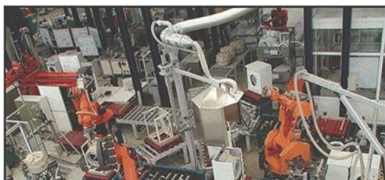
Fig. 3.13 Hybrid system for disassembly of washing machines [19]
