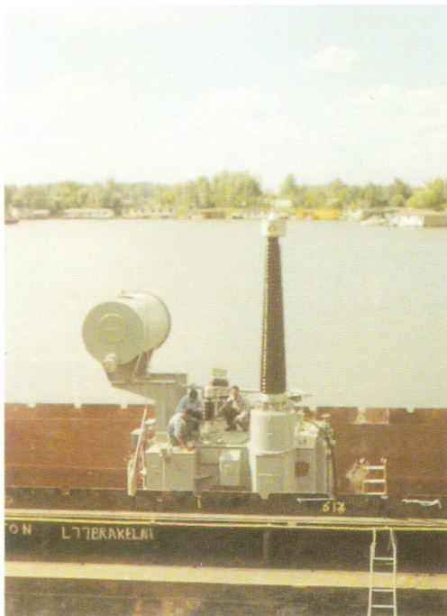
70 MVA Single phase and 186.2 MVA Three phase Transformer on Short Circuit Test barge at KEMA, Netherlands
