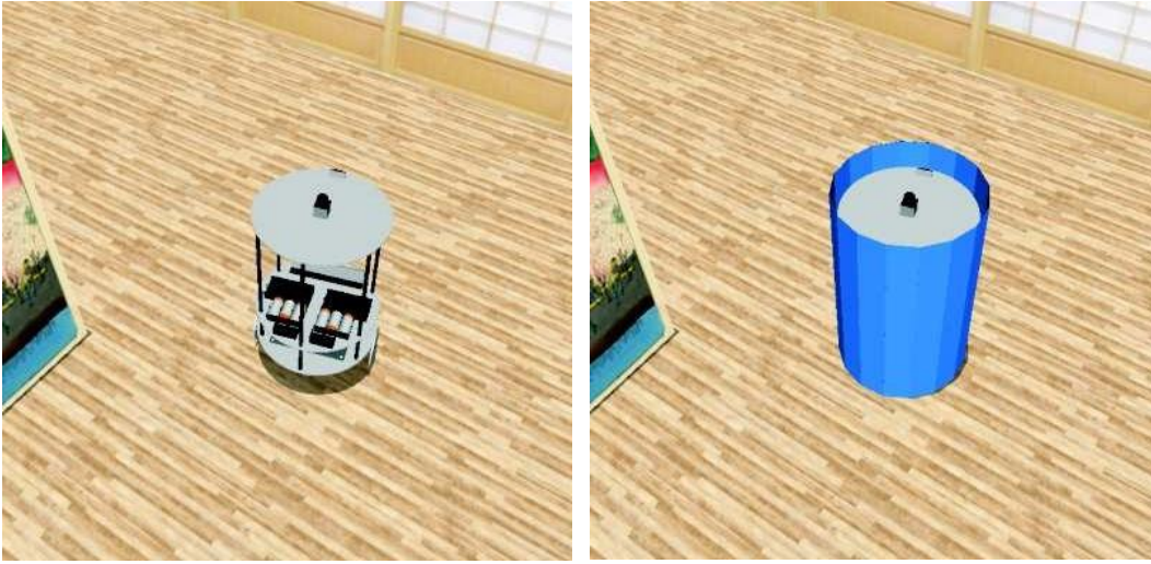
Figure 3.5: Left panel: A simulated robot (from GPRSim), consisting of more than 100 objects. Right panel: An example (in blue) of a collision geometry.
