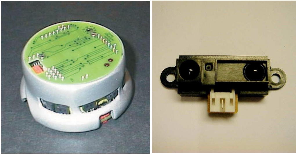
Figure 1.5: Left panel: A Khepera II robot. Note the IR proximity sensors (small black rectangles around the periphery of the robot), consisting of an emitter and a detector. Right panel: A Sharp GP2D12 infrared sensor.
