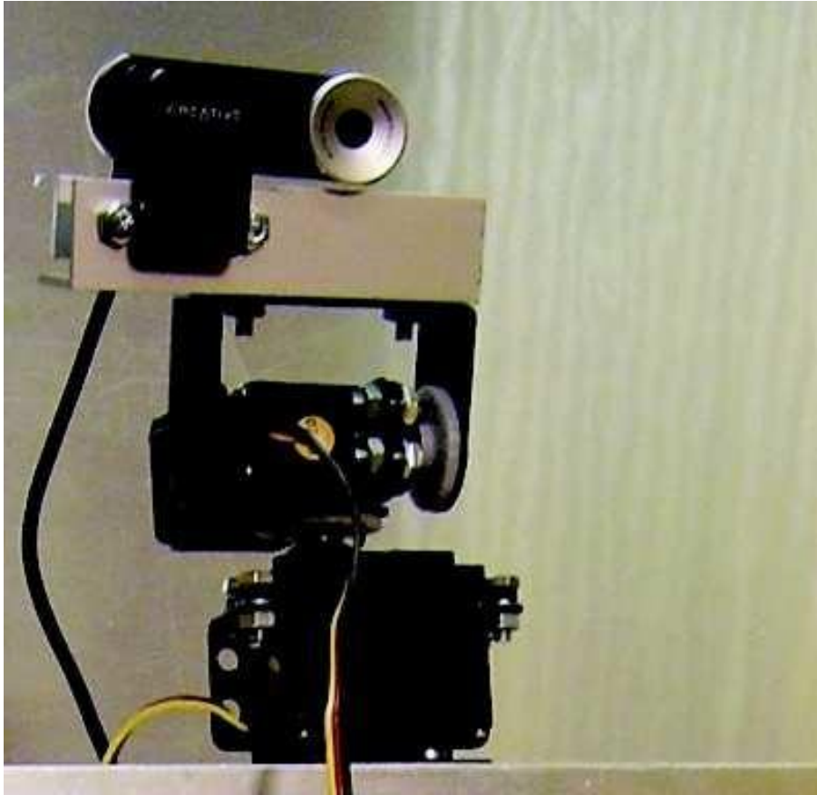
Figure 1.9: A simple robotic head, consisting of two servo motors and a webcam.
